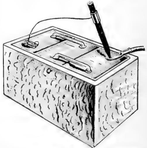
The current taken from the cell is sufficient to weld the connections to the binding-posts
